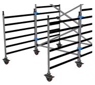
2. Secure each buttress frame to the main tower structure using the approved swivel couplers. 1 above the top rung and 1 above the second rung on each side.
