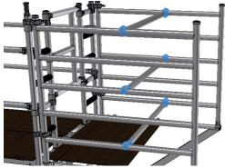
5. From behind the rungs fit an additional set of guardrails on Cantilever frame rungs for the new platform, pushing down to lock on.
