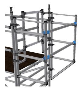
2. From behind your current guardrail or gated frame, fit an additional set of guardrails onto the Cantilever frame rungs for the new platform. Hooks facing outwards.
