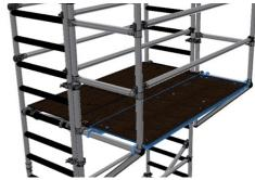
4. From behind the guardrail braces fit a platform next to the infill platform.
