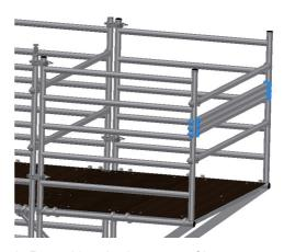
8. Reposition the inner set of braces to store ready for safe dismantling on the tower
