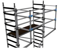
2. From behind the guardrail braces fit 2 more braces to complate a new guardrail.
