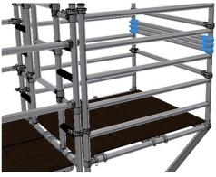
8. Reposition the inner set of braces to store ready for safe dismantling on the tower. (Double Width Cantilever only)
