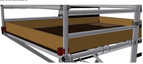
Dismantling is the reverse of assembly. You MUST reposition the stored braces before removing any platforms.
