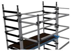
3. From behind the guardrail braces fit the infill platform.
