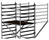
2. Fit cantilever frames; ensure the rungs line up to avoid trip hazards on the platform decks. Ensure couplers are tight. Repeat on the opposite side.
