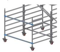
3. Fit 1 buttress horizontal brace to the vertical above the 5th rung and 1 above the of a buttress frame at the furthest point bottom rung at the end away from the main away from the main tower. tower structure
