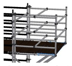
7. From behind the inner set of guardrails fit a platform next to the one you are on. Go to Step 9
