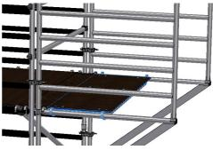
4. From behind the guardrail braces fit a platform next to the infill platform. (Single Width Cantilever go to step 6)
