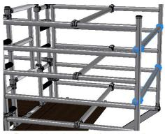
6. Reposition the inner braces to the verticals above the 3rd and 5th rung on the Cantilever frames to complete your working guardrails, hooks facing out.
