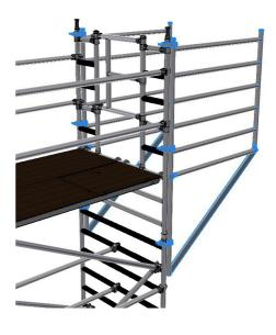
2. Fit cantilever frames; ensure the rungs line up to avoid trip hazards on the platform decks. Ensure couplers are tight. Repeat on the opposite side.
