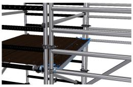
3. From behind the guardrail braces fit the infill platform.
