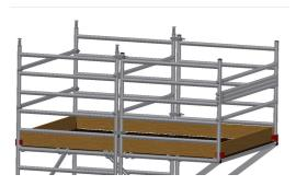
9. Fit toeboard clips and toeboards to complete the structure.
