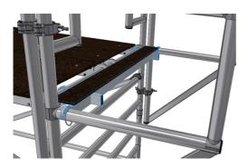
3. From behind the gate fit the end infill platform.
