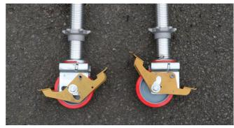
Castor locked (Note castor wheel axle has moved in line with the leg tube)
