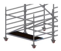
5. Fit ballast platform to the bottom rung at the end away from the main tower structure. Level the buttress using a spirit level as a guide; re-tighten couplers before continuing (if required).
