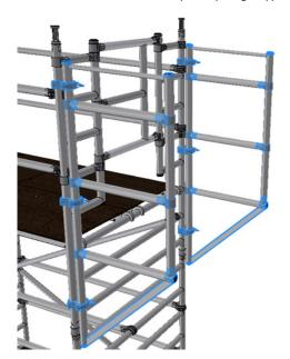
1. Fit 6 swivel couplers to your tower as seen above. Fit cantilever frames; ensure the rungs line up to avoid trip hazards on the platform decks. Ensure couplers are tight. Repeat on the opposite side.
