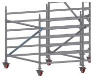
4. Fit 1 diagonal brace to the bottom rung
