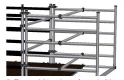
5. Fit an additional set of guardrail braces. This will be 3 horizontal braces hooks facing down to lock onto the cantilever frames.
