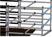
6. Reposition the inner braces to the verticals above the 3rd and 5th rung on the Cantilever frames to complete your working guardrails, hooks facing out.
