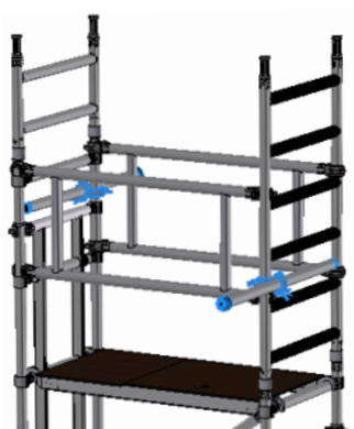
9) Using the method on page 6, fit a side prop to the top of each frame, one either end of the tower above the 3rd rung down. To complete your build go to step 21. If you would like to build higher continue to step 10.
