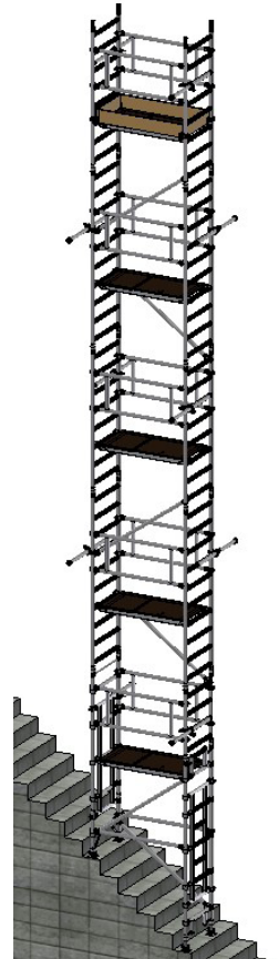
18) Fit a side prop to the top of each frame above the 3rd rung down, one either end of the tower.
