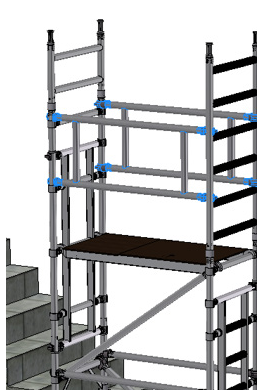
8) Sitting through the platform, fit 2 guardrail frames, one either side or 4 Horizontal braces 2 either side with hooks facing out. Ensure hooks are fully engaged.
