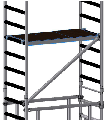
12) Fit a trap platform to the 7th rung down from the top when installing on a FKS5/10.
