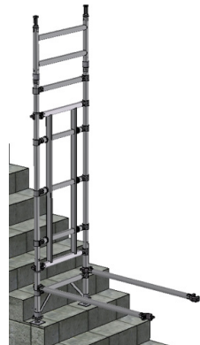
3) Position the plain portal at the top of your stairs then fit the horizontal braces above the 1st rung. The gates should be positioned to open outwards.
