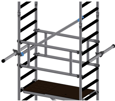
16) Fit a diagonal brace ensuring the top hook lands on the bottom rung of the frame above.
