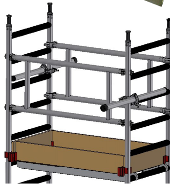
20) Then fit your toe-boards. This can either be a folding toe-board or the blank lengths with clips depending on which kit you choose.
