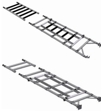
2) Insert a 6 rung SW 232 frame into the 232 gated portal ladder frame and a 2 rung SW 232 frame into the 232 gated portal plain frame. Ensure interlock clips are engaged.
